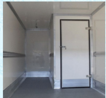
Longitudinal partition wall with door at the end
